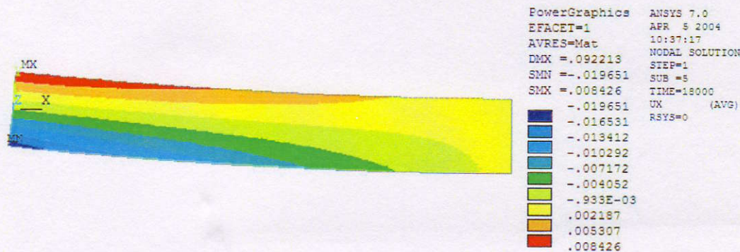
Figure 8. X axis displacement [m] in the concrete beam model after 18 \cdot 10^3 s.
